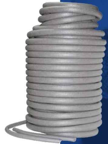
PE cord is a round seal, which fulfils the requirements of the DIN 18450 for backfill material on expanding joints. It consists of closed cellular polyethylene foam and is suitable for sealing against drafts and heat loss. PE cord provides a reliable backfill on building joints and is characterized through its excellent compatibility with all standard sealing materials. Used as a backing support for sealants, 3-sided adhesion can be effectively eliminated.
