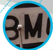
**PARAFUSO AUTOPERFORANTE CHAPA MATRÍCULA**
